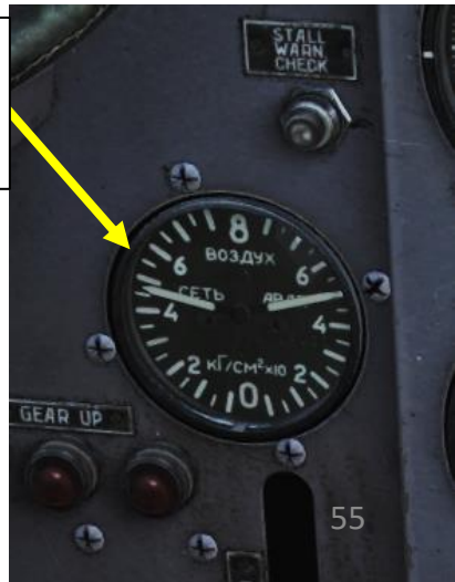
Compressed Air Dual Gauge (x 10 kg/cm²) LEFT: Main Air System Pressure RIGHT: Emergency Air System Pressure
