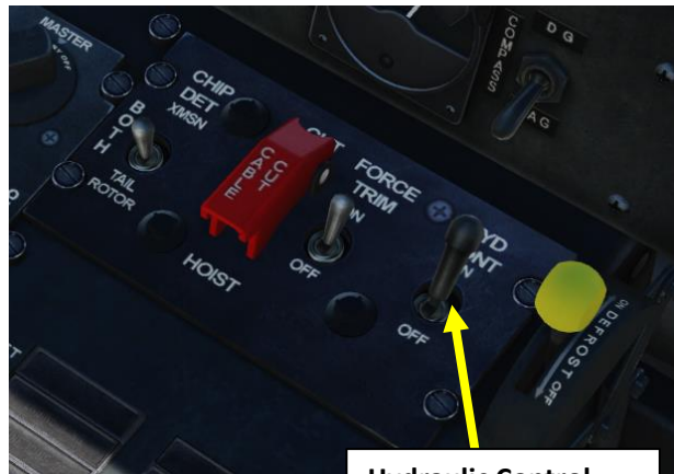
Hydraulic Control (HYD CONT) Switch
