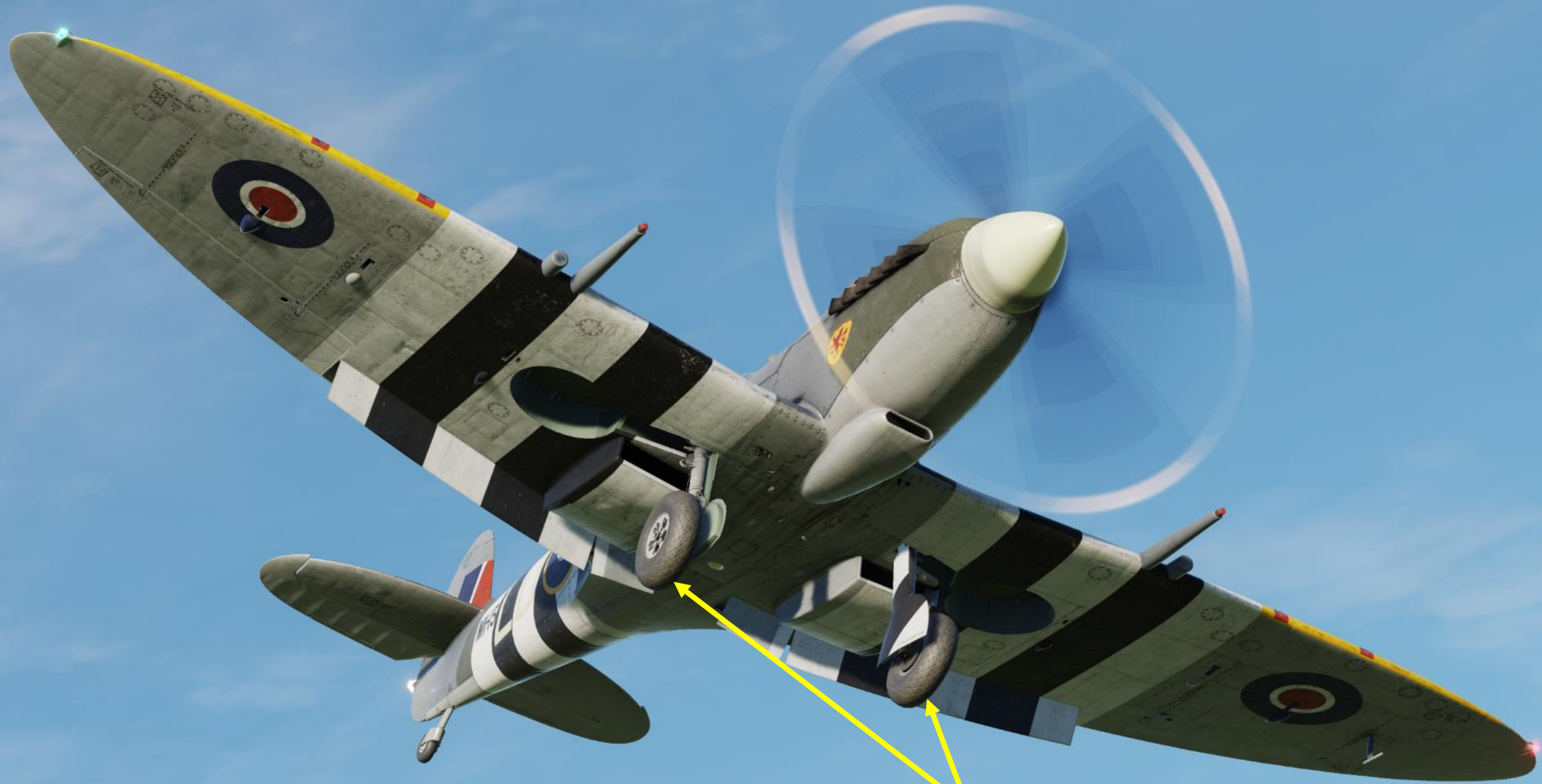
Landing Gear (shown deployed) Hydraulically actuated
