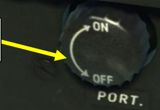
Portside (Left) Flood Lights Control Knob
