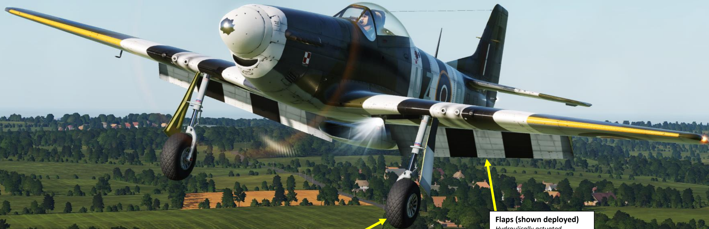
Landing Gear (shown deployed) Hydraulically actuated
