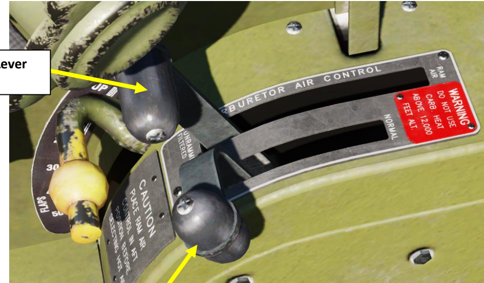
Carburettor Warm Air Control Lever (Hot Air)
