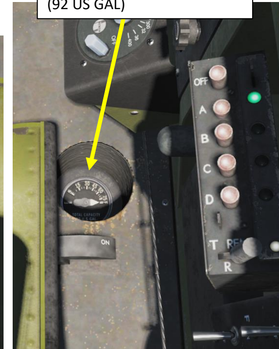
Right Wing Tank Fuel Gauge (92 US GAL)
