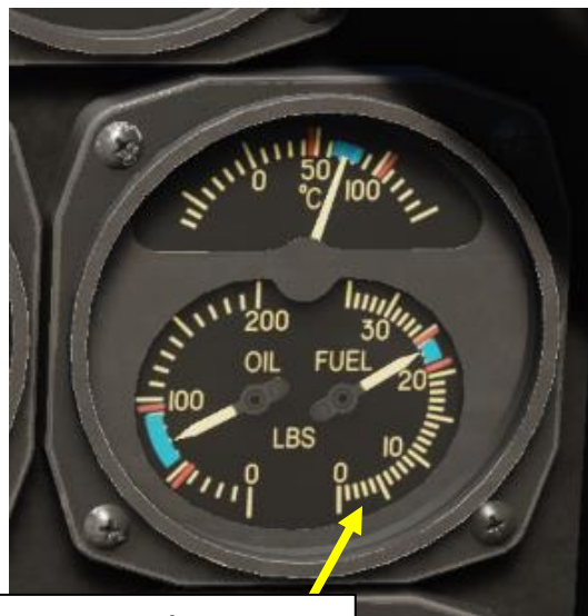
Engine Fuel Pressure Indicator (psi) Blue: Operational Range
