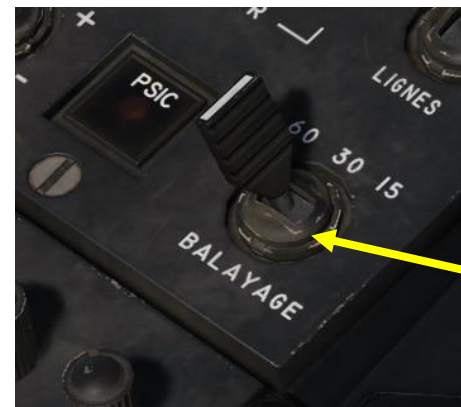
Radar Scan azimuth selector • ( balayage = sweeping angle in degrees, 60/30/15)
