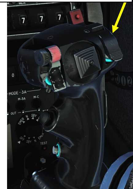
Nav Update / Magic Unlock Button (can be used to switch Magic II Search Mode)
