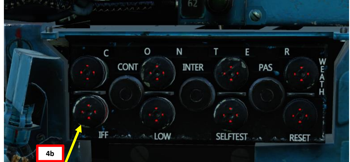
Radar Jamming Filter Button (Interrogation/IFF Mode)
