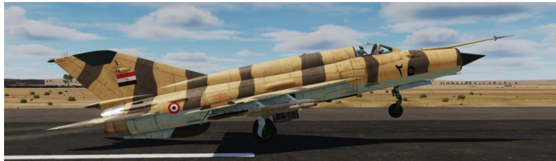
Bad touchdown: slow and high Angle of Attack (20 deg). You are likely to violently smack your tail on the ground.
