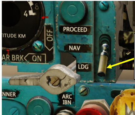
RSBN Mode Selector • UP: Descend (Proceed) Mode • MIDDLE: Navigation Mode • DOWN: Landing Mode
