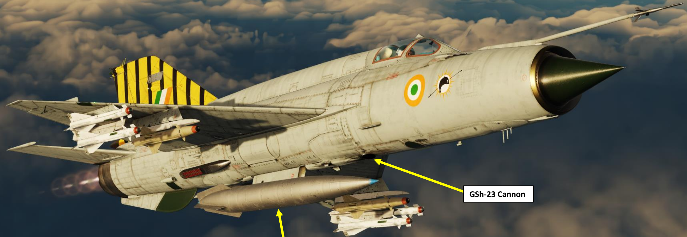
External Fuel Tank
