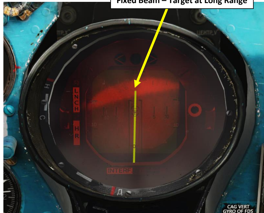
Fixed Beam – Target at Long Range
