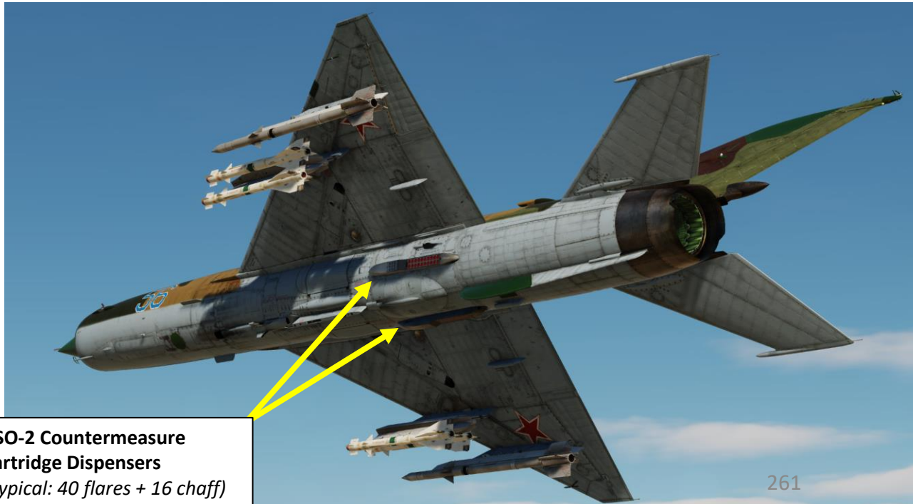
Countermeasure Cartridge Dispensers (Typical: 40 flares + 16 chaff)
