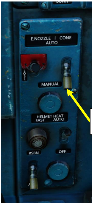
Nose Cone Control Switch • MANUAL
