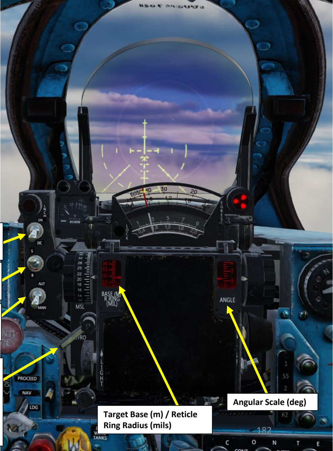
ASP-PFD Optical Sight Mode • UP: Gun • DOWN: Launch (Rockets-Missiles)
