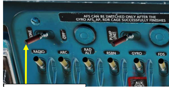
Nose Cone Power Switch • FWD: ON / AFT: OFF
