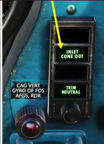
Inlet Nose Cone OUT Light Indicates nose cone is operational. As a general rule, cone should be in only when landing gear is extracted.
