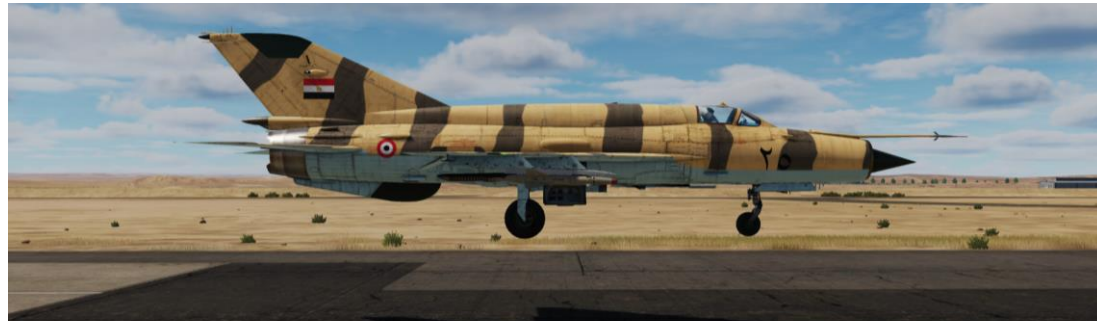
Good touchdown: fast and low Angle of Attack (0-10 deg) – very gentle contact with the ground
