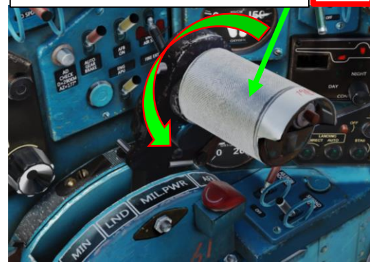
Throttle Twist Grip • Changes ASP Optical Sight Range & Radar TDC Slew Control
