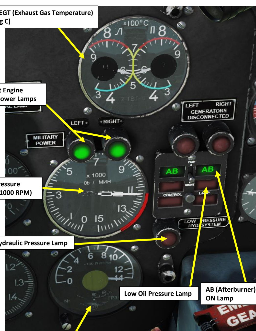
Fuel Flow Meter (x100 Liters/hour)
