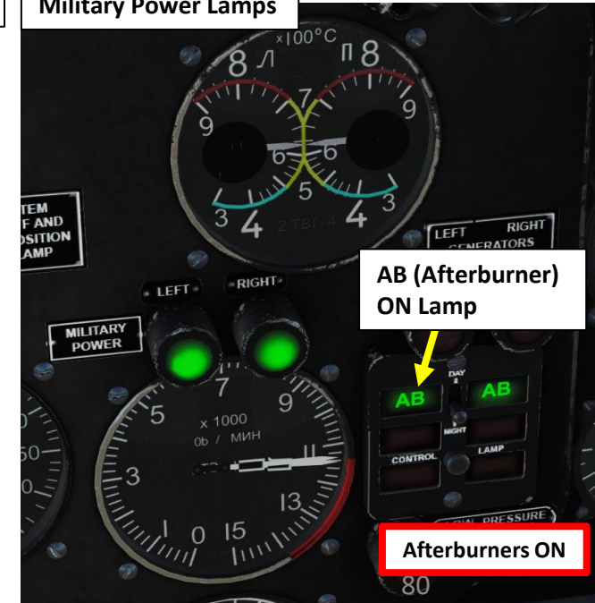
Left/Right Engine Military Power Lamps
