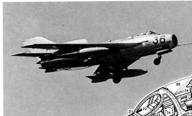
Above: A MIG-19S with undercarriage extended on final approach. The barrel of the massive NR-30 cannon in the starboard wing root may be clearly seen.
