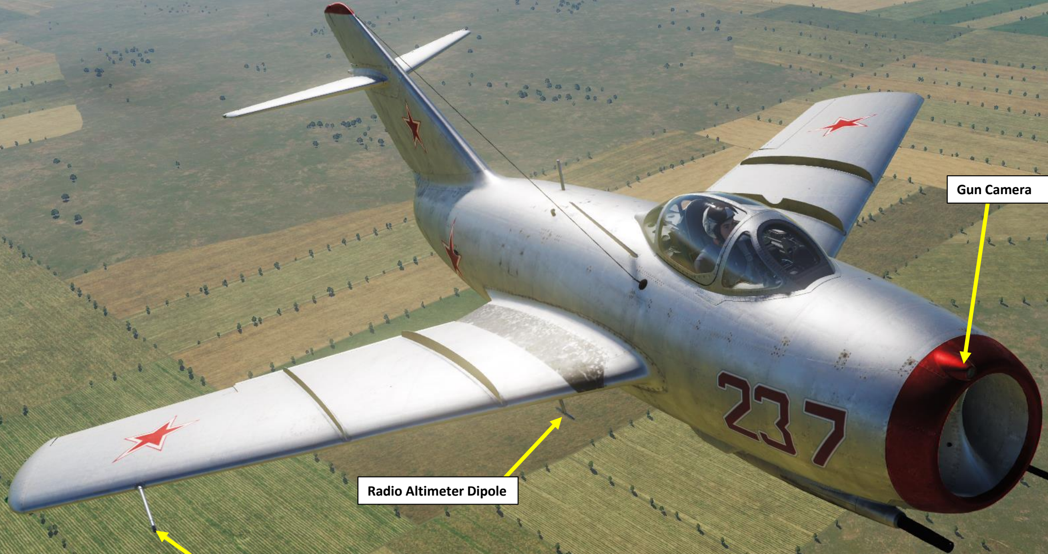
Main Pitot Probe (Pitot-Static) Aircraft of this generation had pretty long pitot tubes in order to avoid the aerodynamic anomalies caused by the air shockwave in front of the wing, which would give erroneous/erratic readings at high speeds. This tube includes both the Pitot Tube (total air pressure) and the static port (static air pressure).
