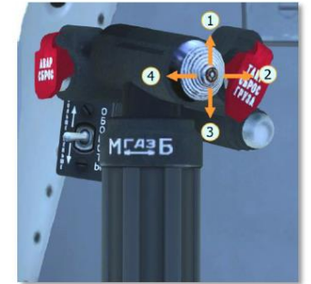
Fig. 7.36. Search/taxi light beam controls
