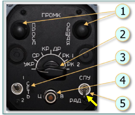
Рис. 9.89. SPU-7 control panel:
