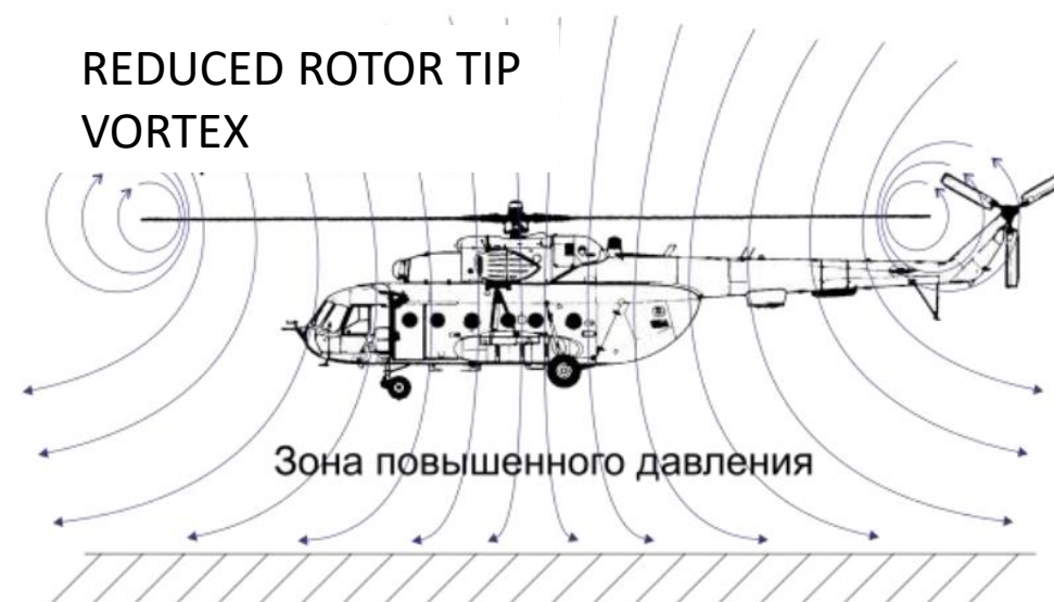
Fig. 9.17. Airflow when in ground effect
