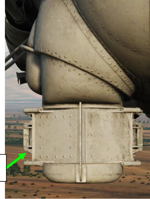
Periscope Outer Doors Closed
