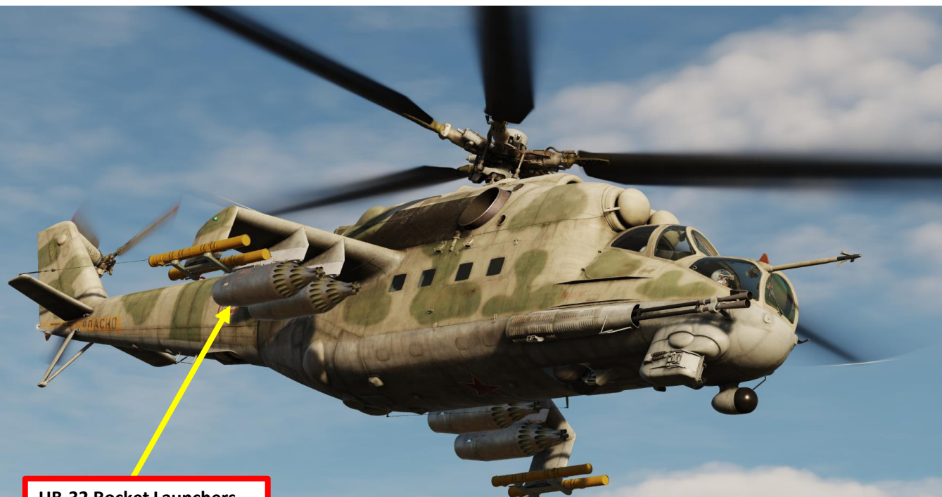
UB-32 Rocket Launchers with S-5 Rockets (x32)
