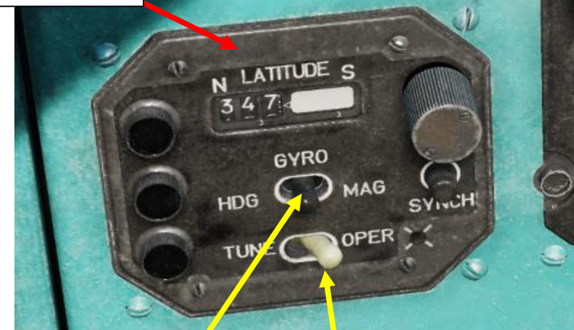
GREBEN-1 Course Control / Flight Director System Control Panel
