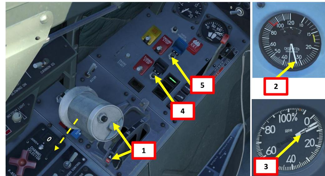
If N1 is lower than 15 %, an **APU-assisted** engine restart is required
