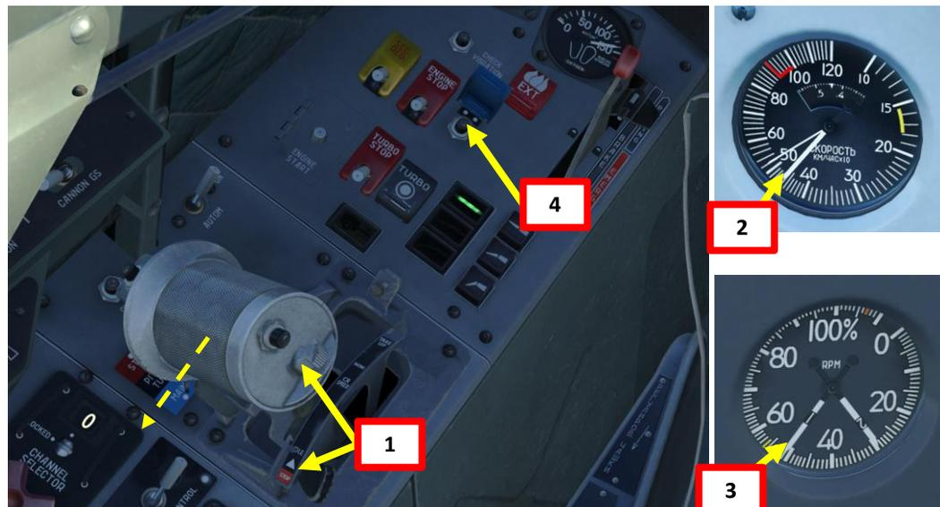
If N1 is higher than 15%, a **windmilling** engine restart can be performed
