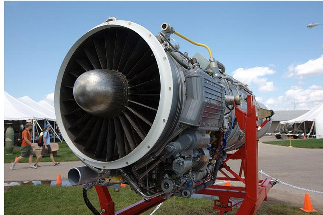
The engine has a JPT (Jet Pipe Temperature) regulator, which is basically an EGT (Exhaust Gas Temperature) overheat protection system. This automated controller will regulate fuel flow sent to the combustion chamber to avoid damaging the engine.
