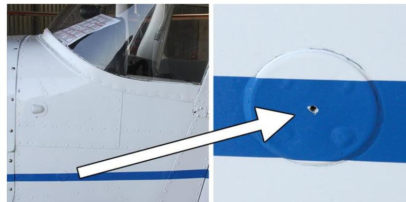
The static port pressure sensor will feel the pressure of the air laterally (or from the side of the aircraft), but will not feel the dynamic pressure created by the motion of the aircraft. See the “dog in car” analogy from previous page. 84
