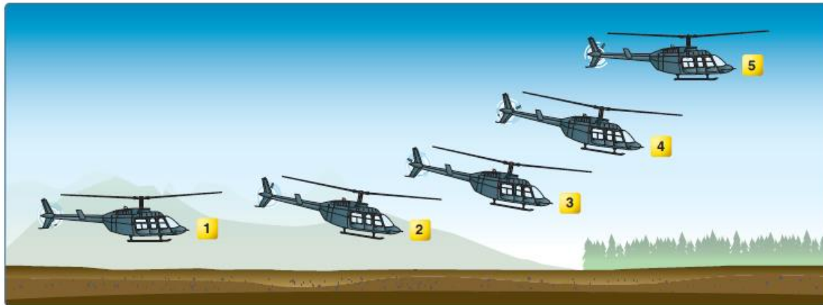
Figure 9-7. The helicopter takes several positions during a normal takeoff from hover.
