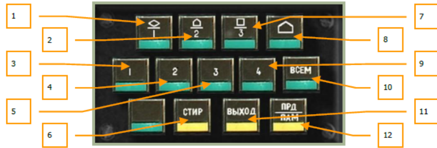
6-32: Data link control panel
