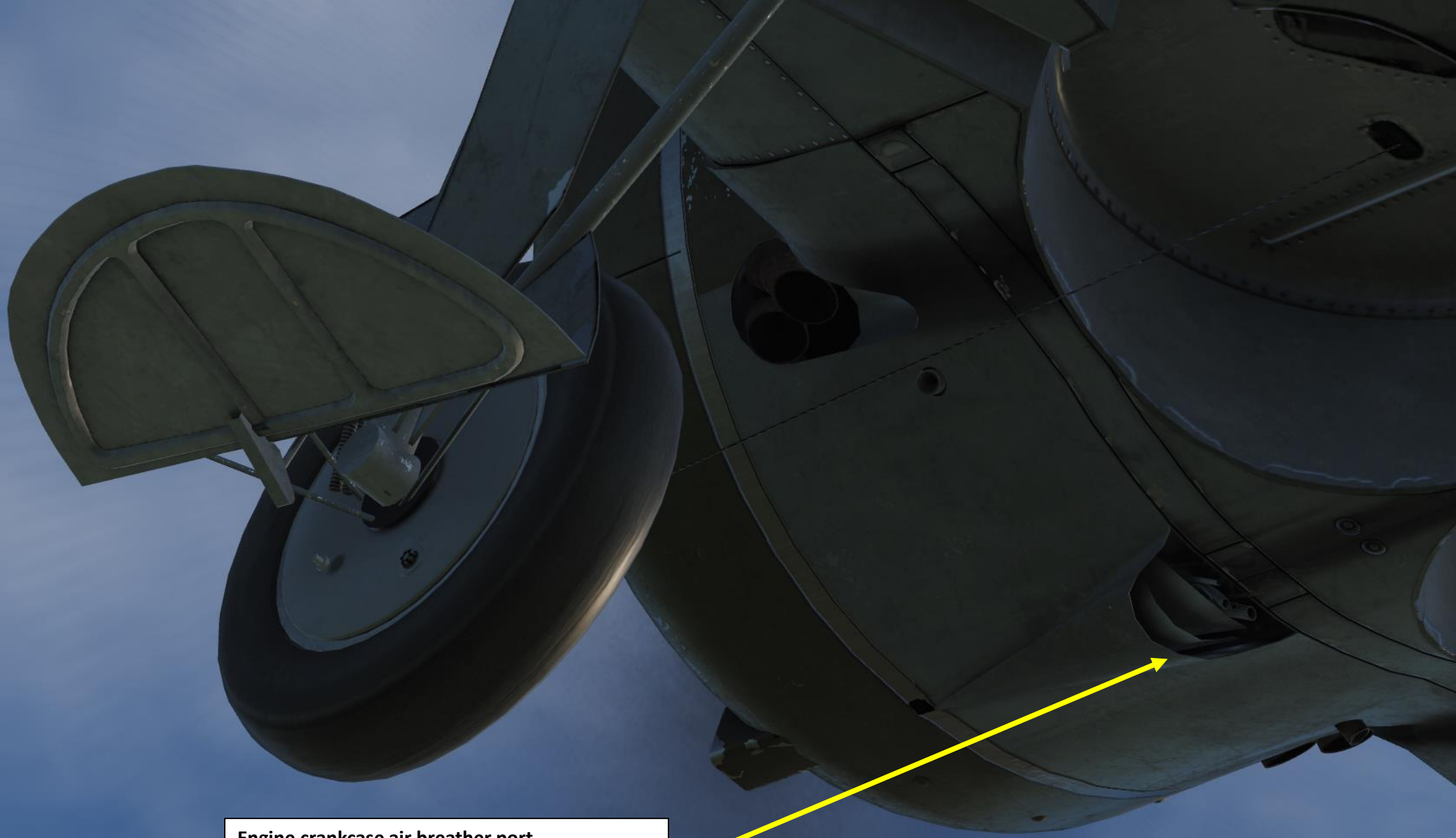
Engine crankcase air breather port Part of the engine crankcase breathing system, which comes from the oil air separator. After high G manoeuvres, a significant amount of oil can come out of this port.
