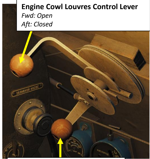
Engine Oil Cooler Control Lever Fwd: Open Aft: Closed
