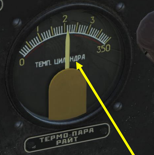
CHT (Cylinder Head Temperature) Indicator (x100 deg C)
