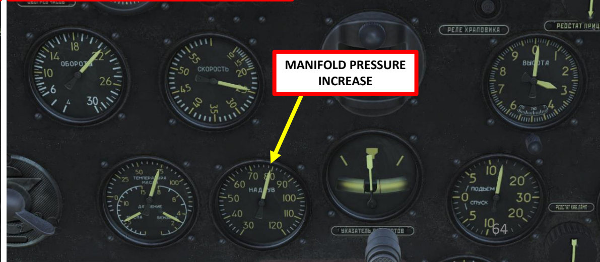
SUPERCHARGER IN SECOND GEAR ALTITUDE: 3000 M
