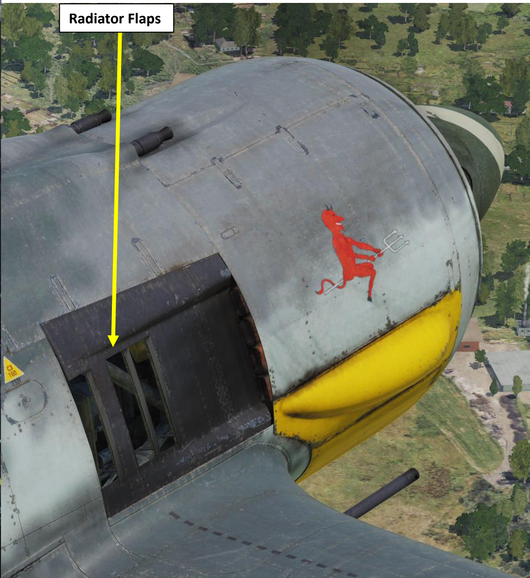
Radiator Flaps Position Indicator Up: Zu (Closed) Down: Auf (Open)
