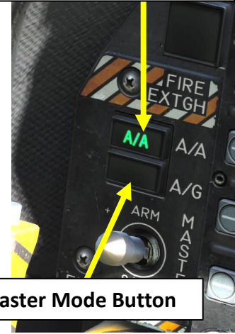
A/A (Air-to-Air) Master Mode Button
