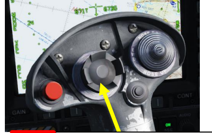
9a Sensor Control Switch AFT/FWD/LEFT/RIGHT
