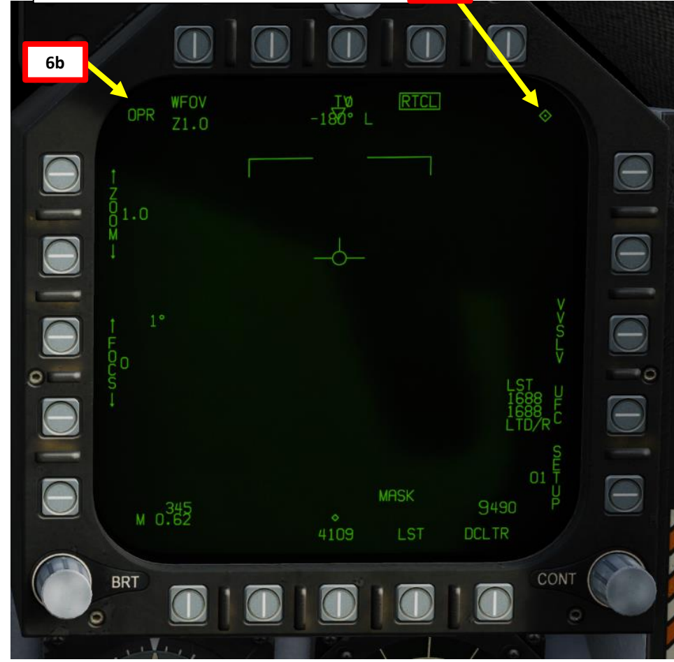
TDC (Throttle Designator Controller) Focus Diamond (TDC is active on this display)
