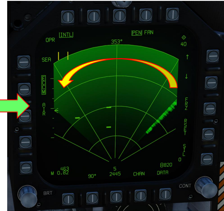
Interleaved Scanning – SEA Displayed
