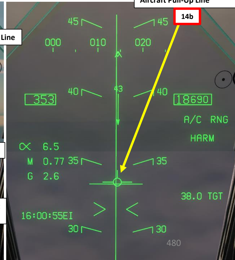
Velocity Vector intersects Aircraft Pull-Up Line
