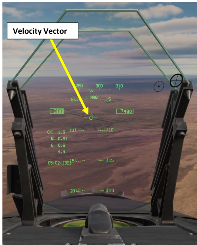
TGP slaved to Velocity Vector (Reticle Shown)
