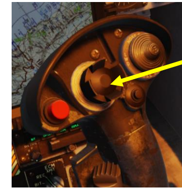
Sensor Control Switch AFT/FWD/LEFT/RIGHT
