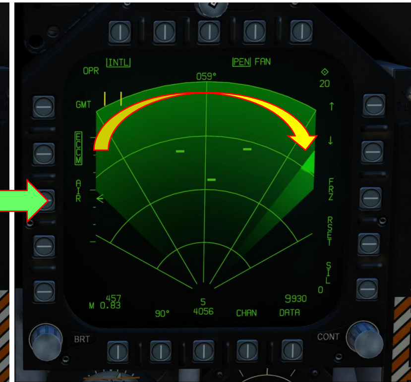
Interleaved Scanning – GMT Displayed
