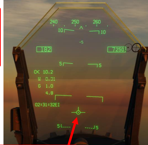
Center Dot on the TVV (Total Velocity Vector) means that the TDC (Throttle Designator Controller) is assigned to the HUD
