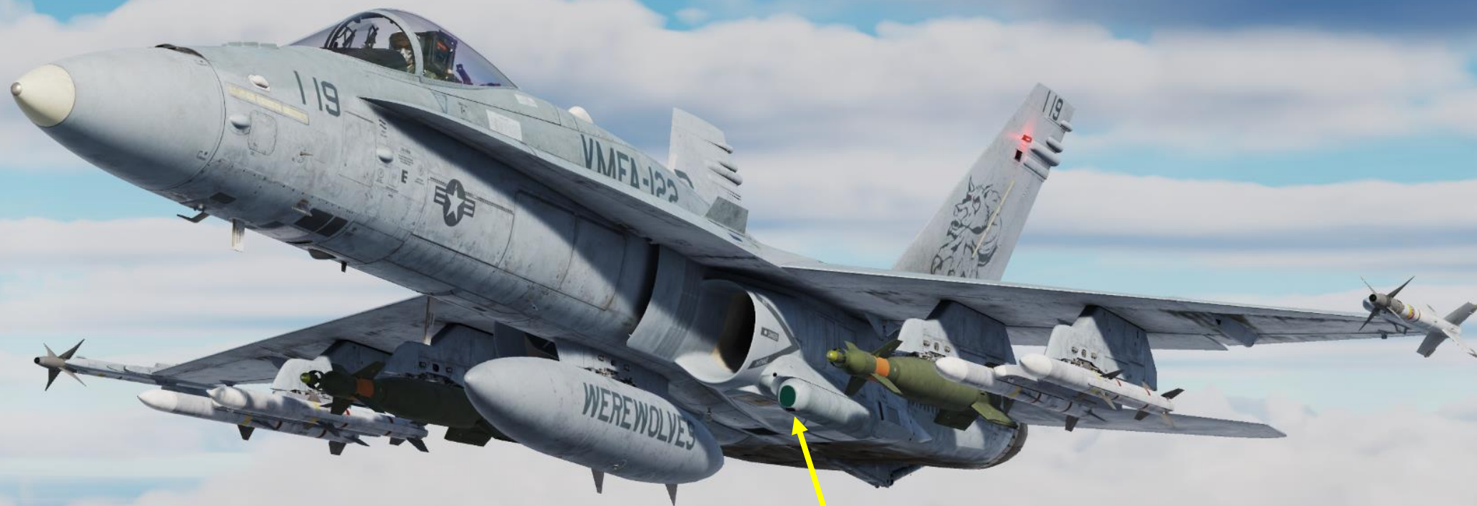
ATFLIR Targeting Pod
