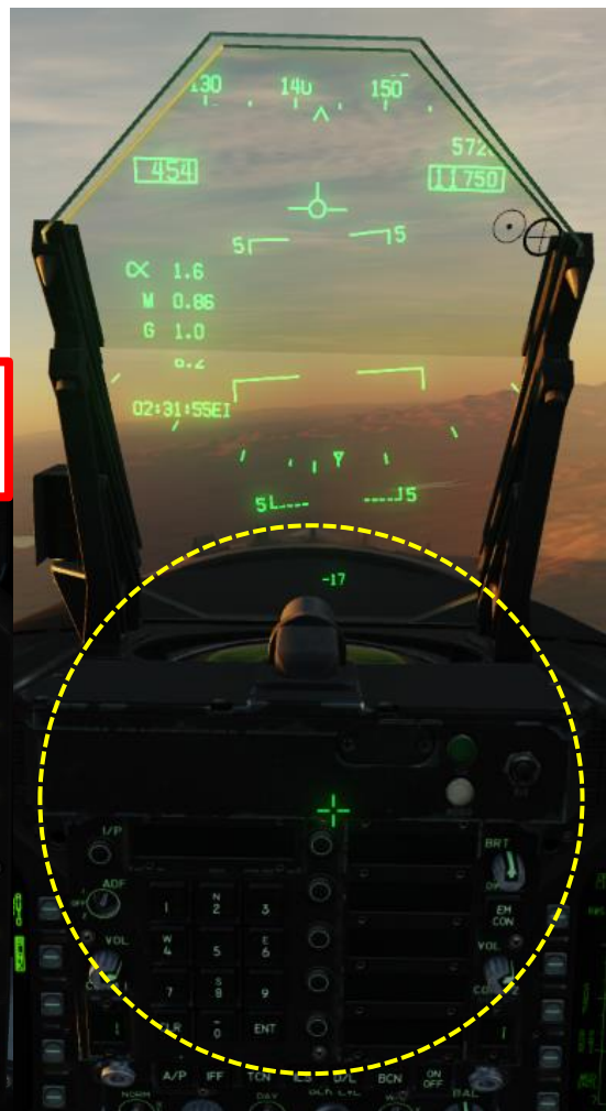
Automatic Blanking (HMD Occluded on HUD)
