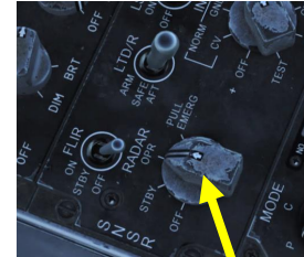
Radar Power Switch
