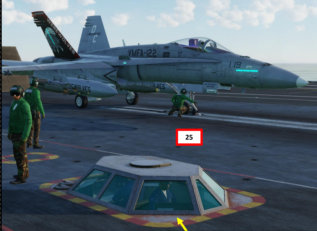
Integrated Catapult Control Station (ICCS), also called “The Bubble”.
