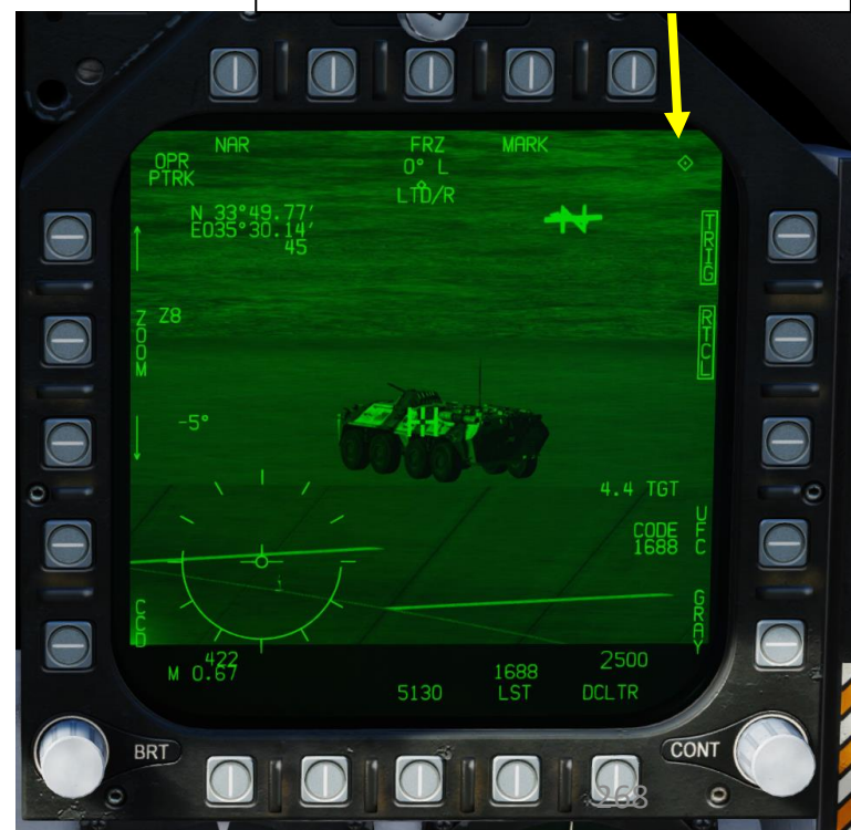
TDC (Throttle Designator Controller) Focus Diamond (TDC is active on this display)
