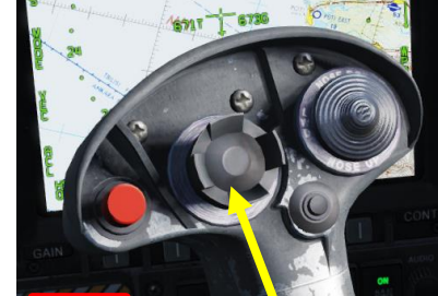
9a Sensor Control Switch AFT/FWD/LEFT/RIGHT
