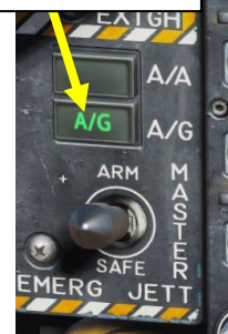
A/G Master Mode Button (required to use laser)
