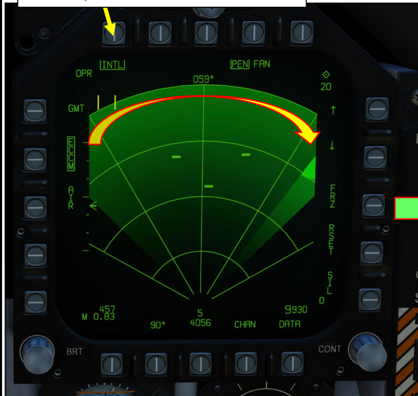
Interleaved Scanning – GMT Displayed
