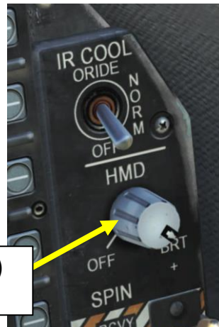
HMD (Helmet-Mounted Display) Brightness Control Switch
