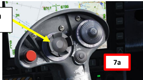
Sensor Control Switch AFT/FWD/LEFT/RIGHT
