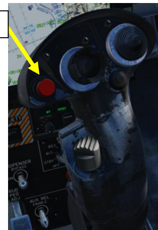
Scenario: Pullback Mode is inhibited. Weapon Release button is pressed: No HARM is launched.
