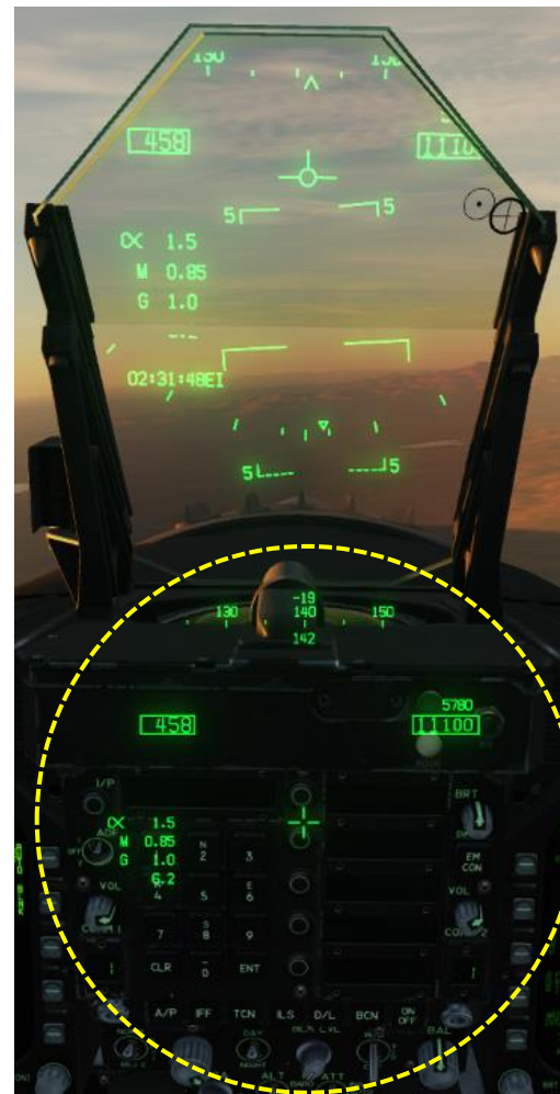
Manual Blanking (HMD Not Occluded on HUD)
