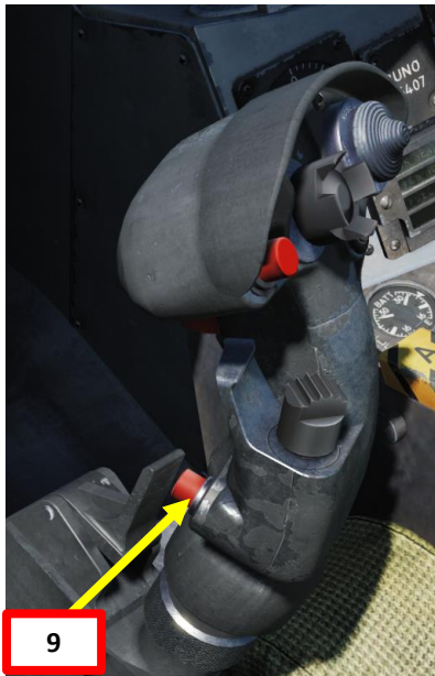
Undesignate / Nosewheel Steering Button
