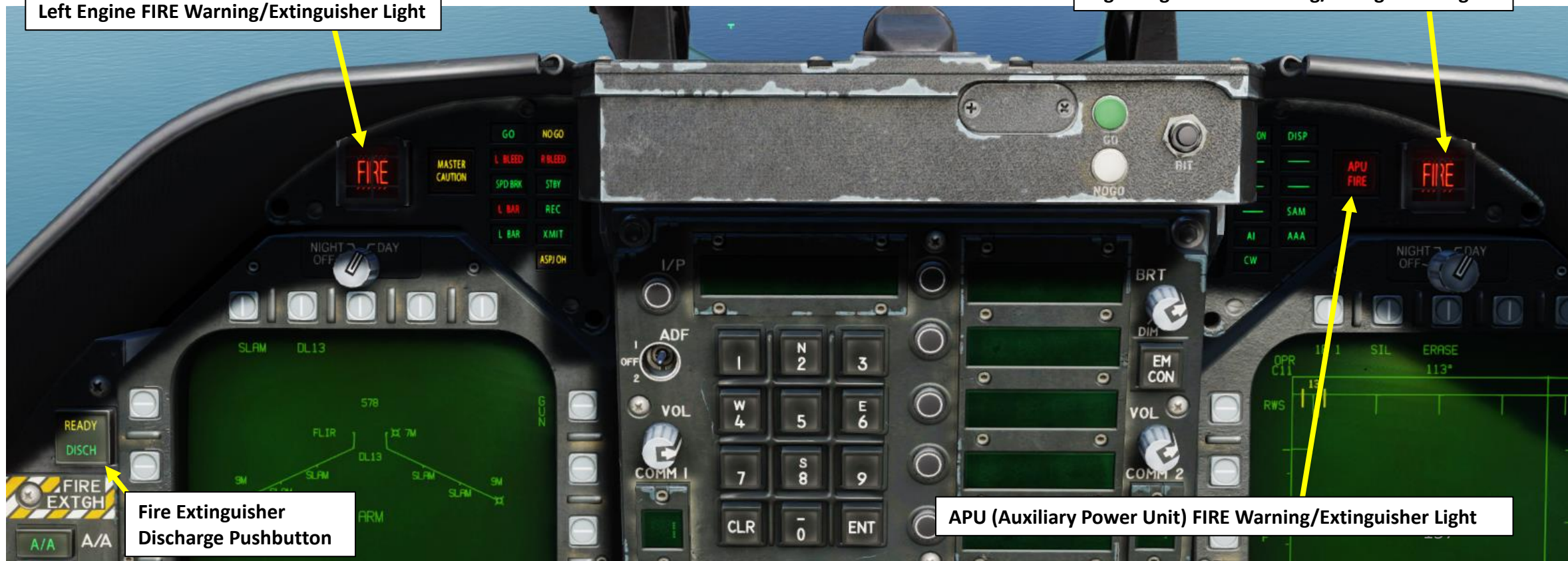
Right Engine FIRE Warning/Extinguisher Light
