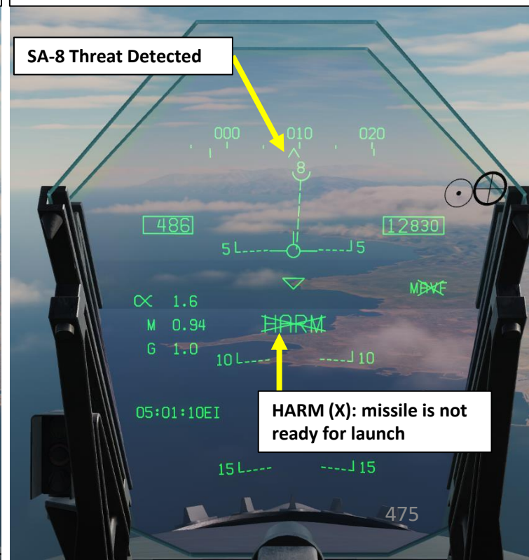
Scenario: Pullback Mode is inhibited. Weapon Release button is pressed: No HARM is launched.
