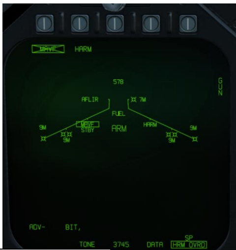
HRM OVRD Boxed: Pullback Mode Inactive
