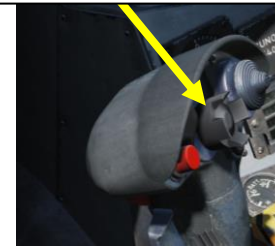
4a Sensor Control Switch AFT/FWD/LEFT/RIGHT
