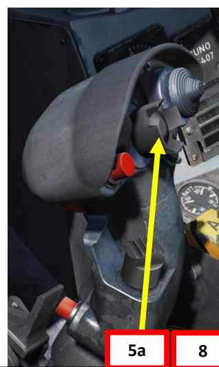
Sensor Control Switch AFT/FWD/LEFT/RIGHT/DEPRESS
