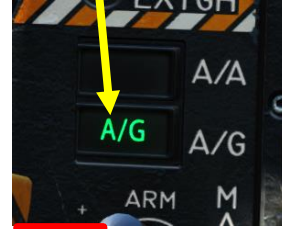
A/G (Air-to-Ground) Master Mode Selected
