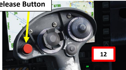
Throttle Designator Controller AFT/FWD/LEFT/RIGHT/DEPRESS
