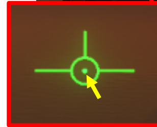
Center Dot on the TVV (Total Velocity Vector) means that the TDC (Throttle Designator Controller) is assigned to the HUD
