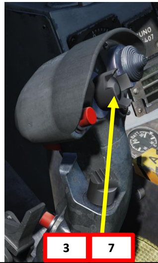
Sensor Control Switch AFT/FWD/LEFT/RIGHT/DEPRESS
