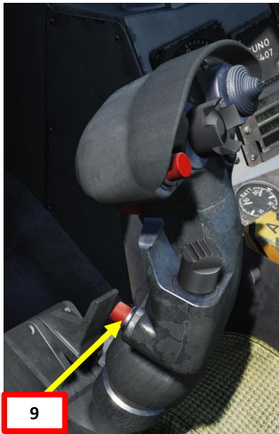
Undesignate / Nosewheel Steering Button
