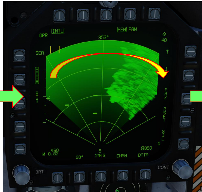
Interleaved Scanning – MAP Displayed
