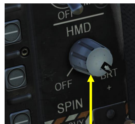
HMD (Helmet-Mounted Display) Brightness Control Switch
