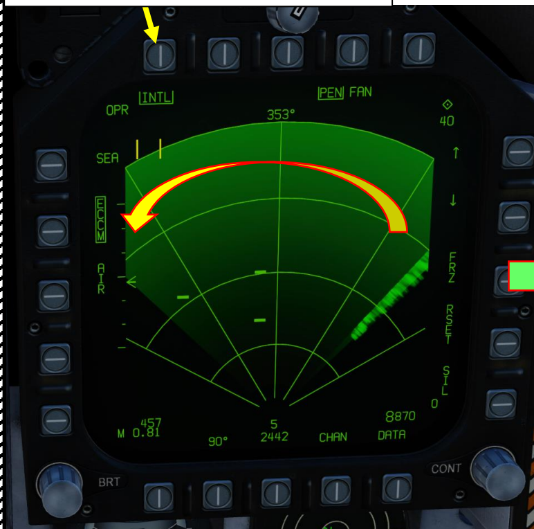
Interleaved Scanning – SEA Displayed
