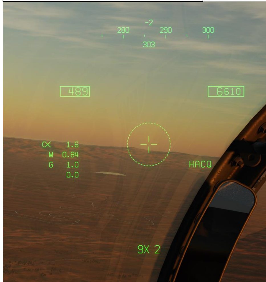
No STT (Single Target Track) Lock Acquired
