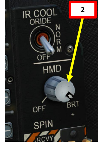
HMD (Helmet-Mounted Display) Brightness Control Switch
