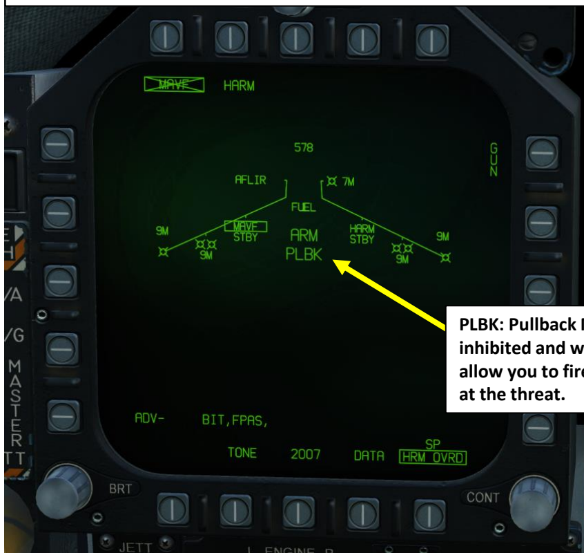
Scenario: Pullback Mode is inhibited and a critical threat is detected. Weapon Release button is not pressed.
