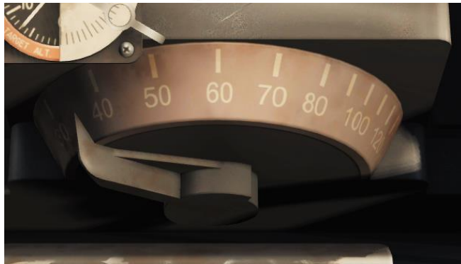
WINGSPAN OF A MIG-15BIS 10 m = 32 ft (VALUE TO ENTER IN GUNSIGHT WINGSPAN)
