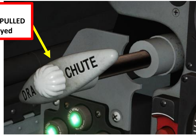
12d Drag Chute Handle – IN Reset Position
