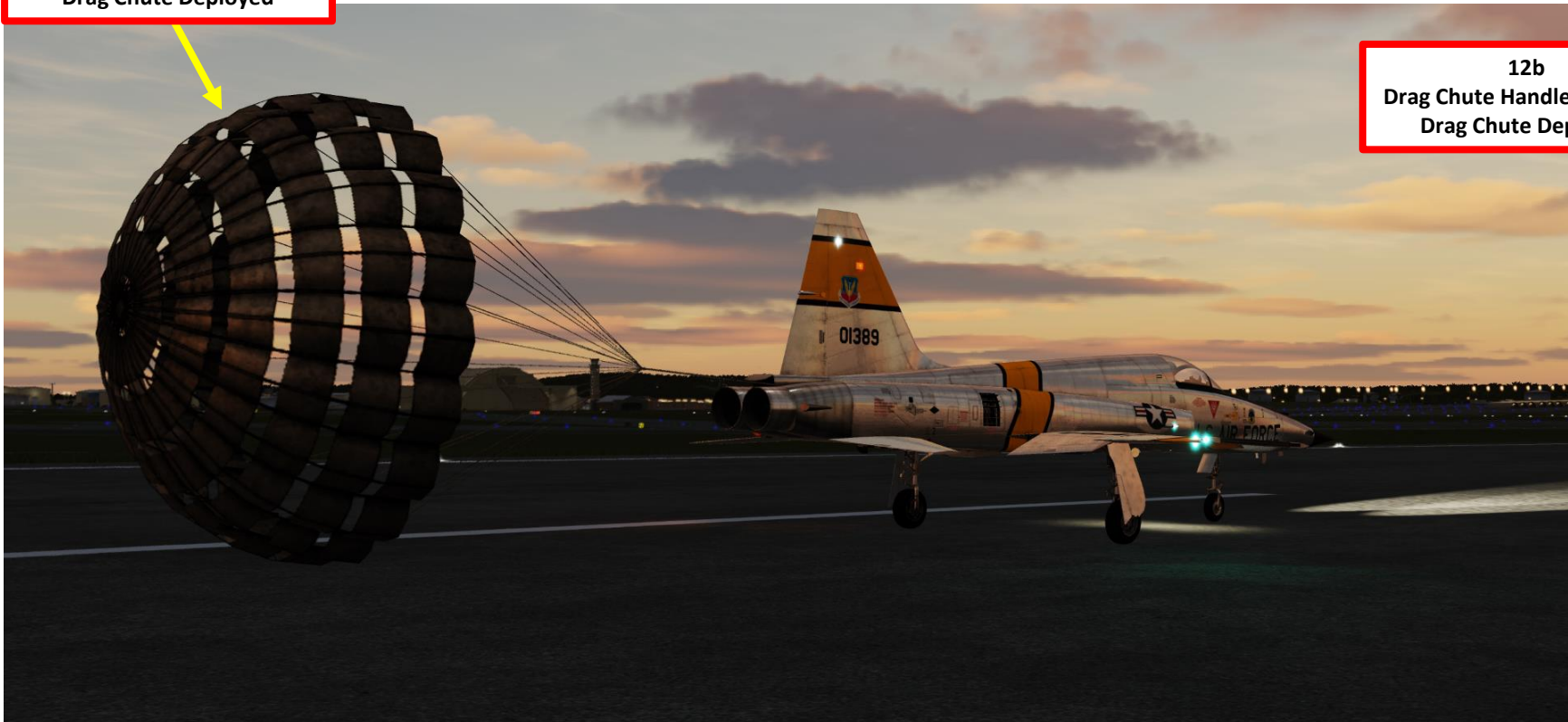
12c Drag Chute Handle – TURNED & PULLED Drag Chute Released
