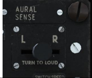
Loop Antenna at 040 Switch Neutral No Sound Audible
