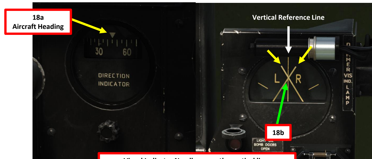
Visual Indicator Needles cross the vertical line. Radio Emitter is straight ahead
