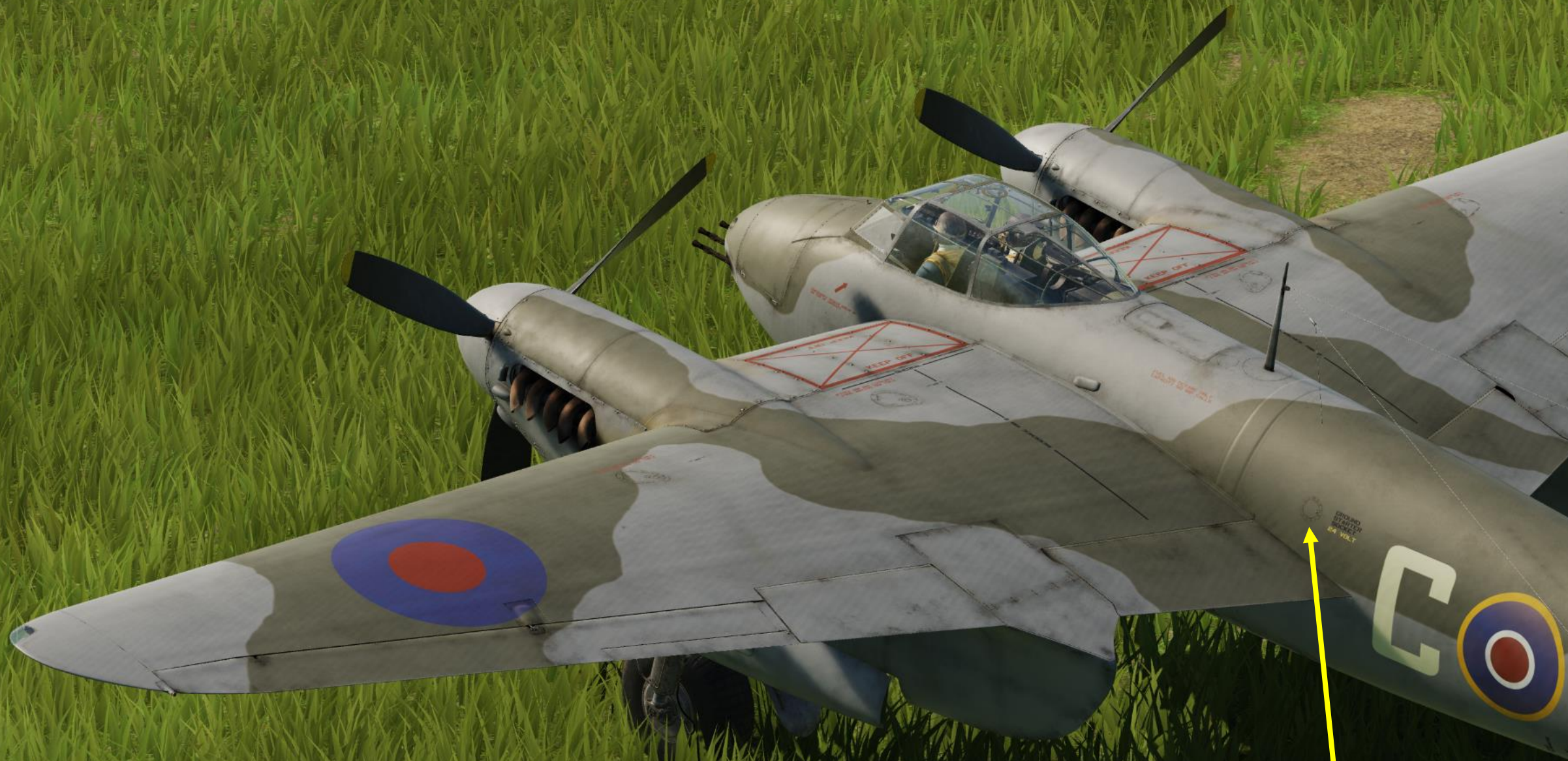
Ground Power Socket (24 Volts)
