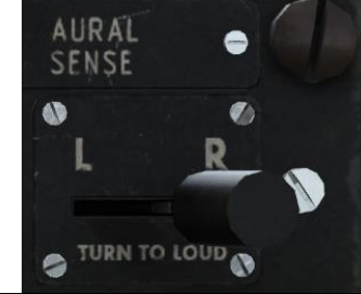
Loop Antenna at 040 Switch RIGHT No Sound Audible No need to turn antenna RIGHT
