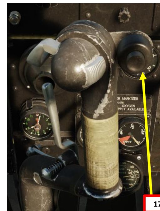
Bomb Release & Gun Camera (Guncam) Button • RSHIFT+SPACE The function of the button depends of the position of the Bombs or Camera Changeover Switch
