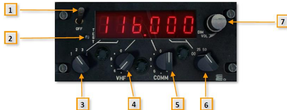
AN/ARC-134 VHF Radio Control Panel
