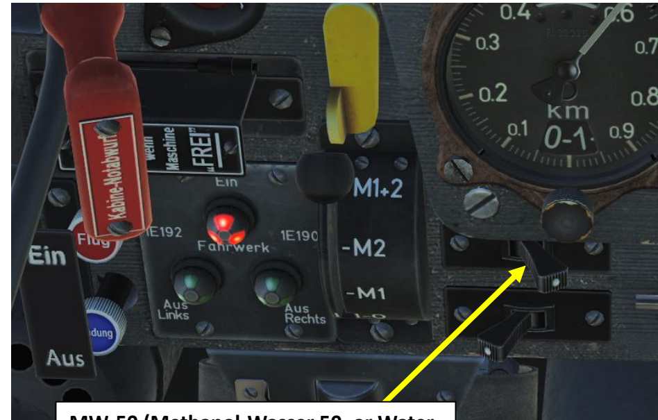
MW-50 (Methanol-Wasser 50, or Water-Methanol Injection) Switch Left = Disabled Right = Enabled
