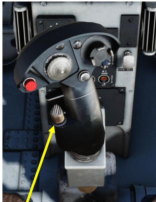
Air-to-Air Weapon Select Switch AFT = A/A Sidewinder SEAM Mode FWD = A/A Sidewinder Boresight Mode DOWN (PUSHED) = Gun Mode
