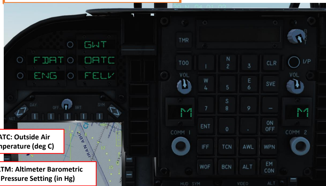
STO Page – Interface with UFC (Up-Front Controller)
