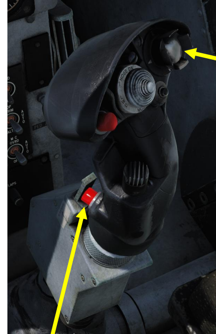
Air-to-Ground Target Undesignate / Nosewheel Steering Button
