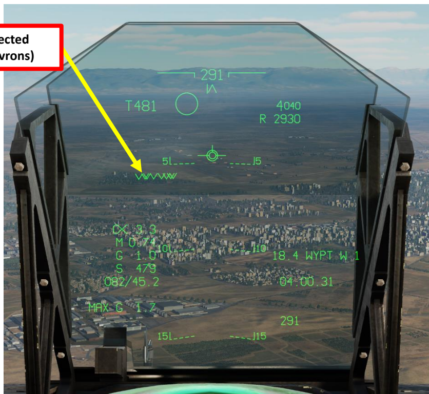
8 x Tanks Detected (Hot Spot Chevrons)
