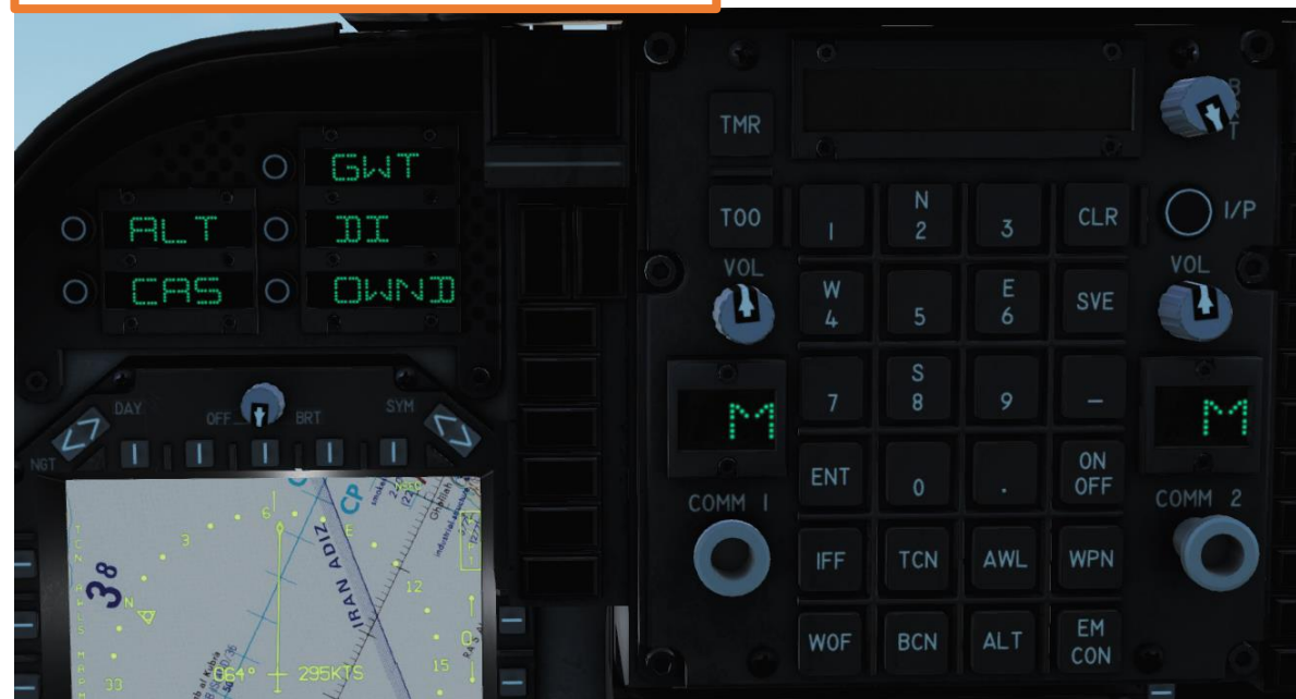
CRUS Page – Interface with UFC (Up-Front Controller)
