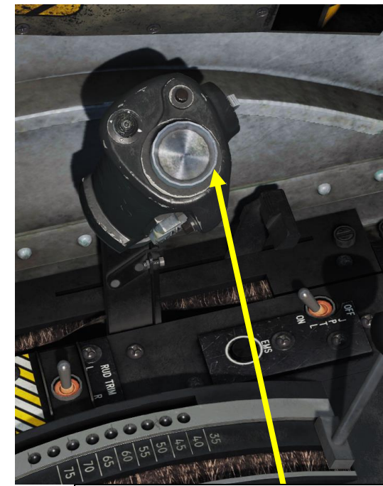
TDC (Target Designation Caret) Control Switch • LEFT • RIGHT • FORWARD • AFT • DOWN (ACTION)
