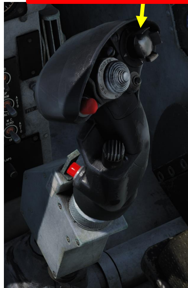
27b Sensor Select Switch (SSS)
