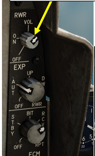
RWR (Radar Warning Receiver) Control Knob OFF / ON / Volume
