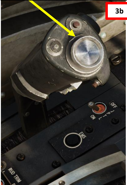
TDC (Target Designation Caret) Control Switch LEFT/RIGHT/FORWARD/AFT/DOWN (ACTION)
