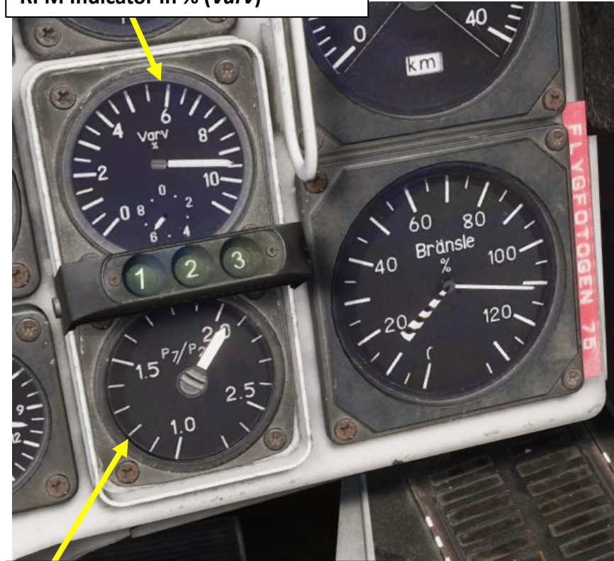
Engine Pressure Ratio (EPR) Indicator (Pt7/Pt2, or ratio between engine intake and exhaust pressures)
