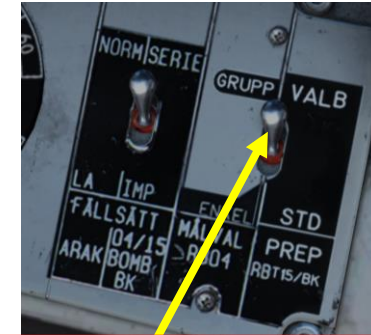
Targeting Mode (MÅLVAL) / Preparation Switch VALB: Program Selectable
