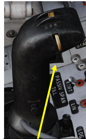
Radar Fix Trigger 15a • T0: Neutral • T1: First trigger detent • TV: Second trigger detent
