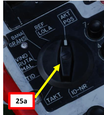
25a Radar Mode Selector A0: Radar OFF A1: Radar ON, Sector PPI
