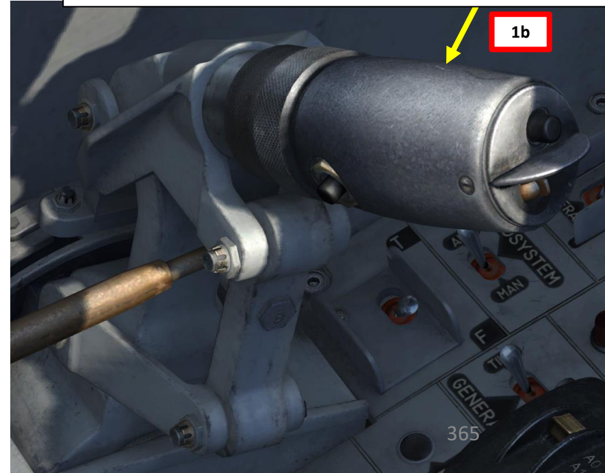
Autothrottle (AFK, or Automatisk Fart Kontroll ) Quick Disconnect Button / Infrared Missile Quick Select Button (In Front of Throttle, Not Visible)
