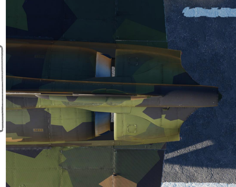
Thrust Reverser System (seen from above)
