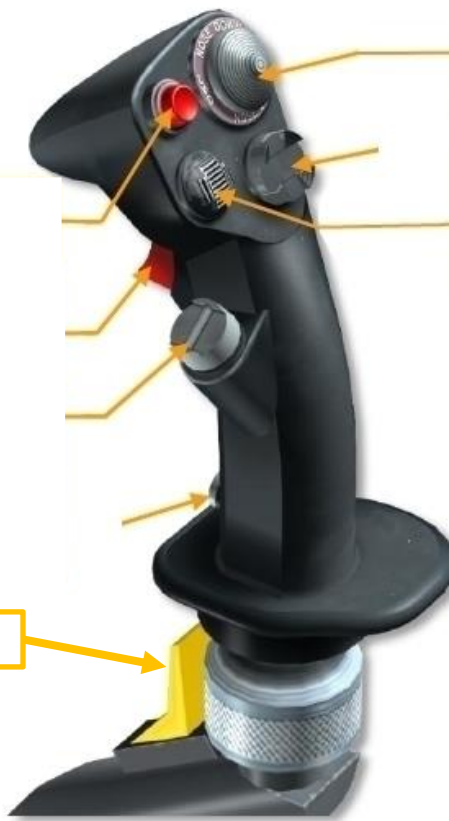
Countermeasures Mode Selector (KB) 0: Off 1: Mode 1 2: Mode 2 3: Mode 3
