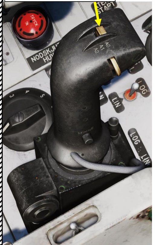
Radar Mode Selector – A0 OFF
