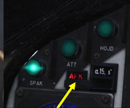
Autothrottle (AFK) Light • Illuminated once autothrottle is in use
