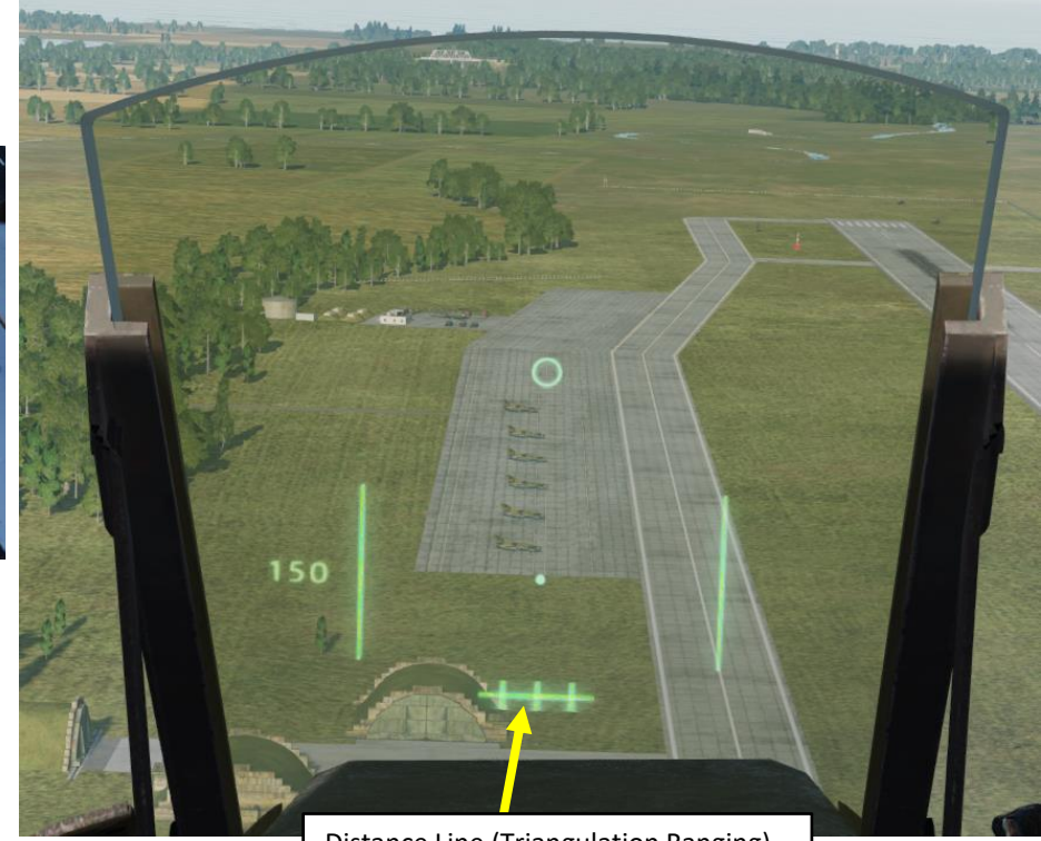
Distance Line (Triangulation Ranging)
