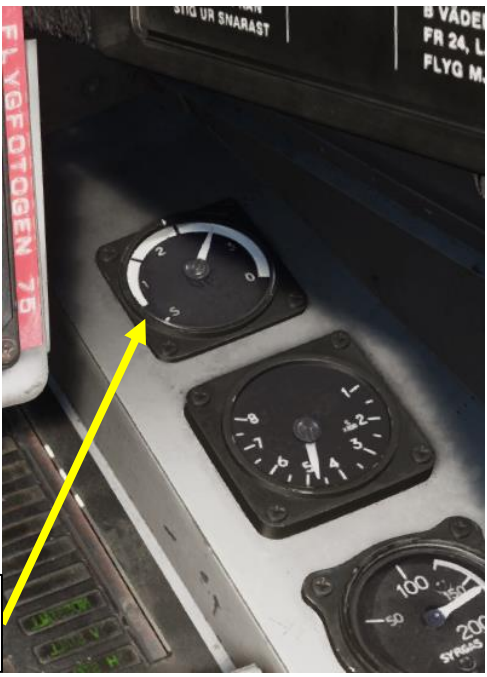
Engine Nozzle Position Indicator (Shown: Afterburner Stage 3)
