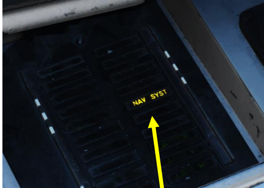
NAV SYST: Navigation System Failure/Malfunction
