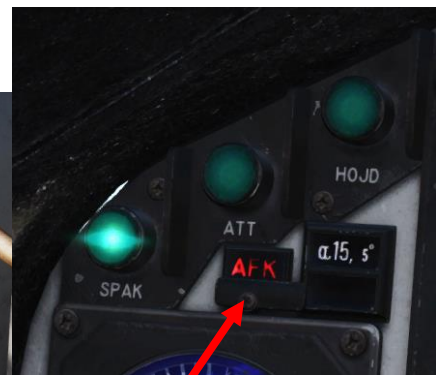
Autothrottle (AFK) Light • Illuminated once autothrottle is in use
