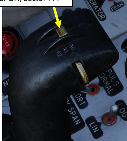
Radar Mode Selector A1: Radar ON, Sector PPI
