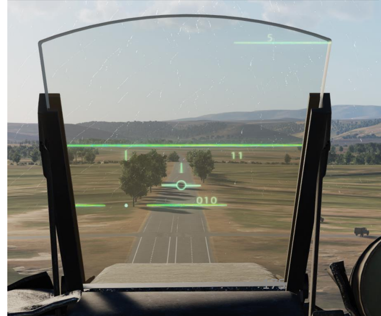
HUD (Heads-Up Display) in LANDN NAV – Prior to Touchdown
