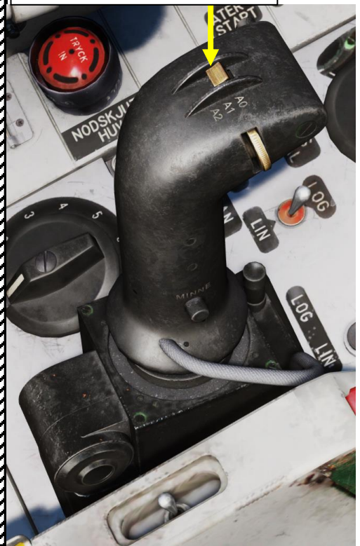
Radar Mode Selector – A2 (Narrow Search with B-Scope)
