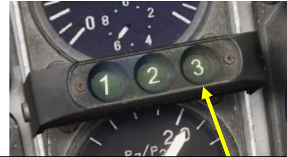
Afterburner Stage/Zone Indicator Lights
