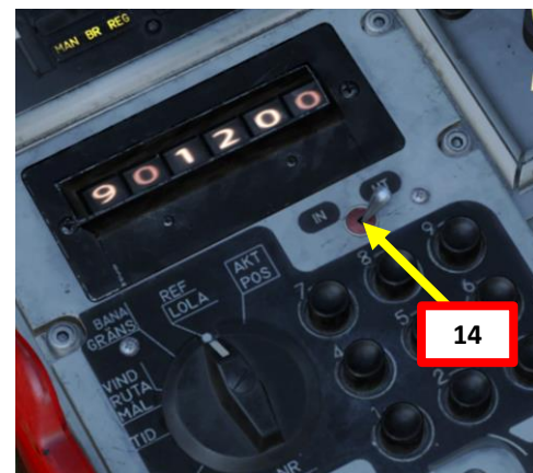
13c All digits set to 0 DATA TRANSFER COMPLETE
