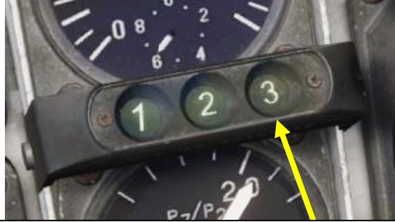
Afterburner Stage/Zone Indicator Lights
