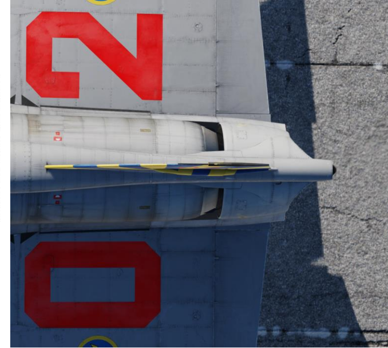
Thrust Reverser System (seen from above)
