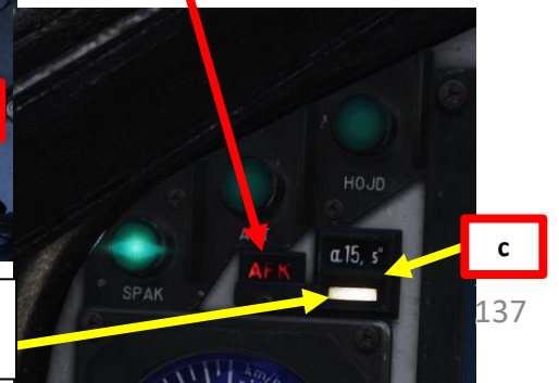
Autothrottle (AFK) Light • Illuminated once autothrottle is in use
