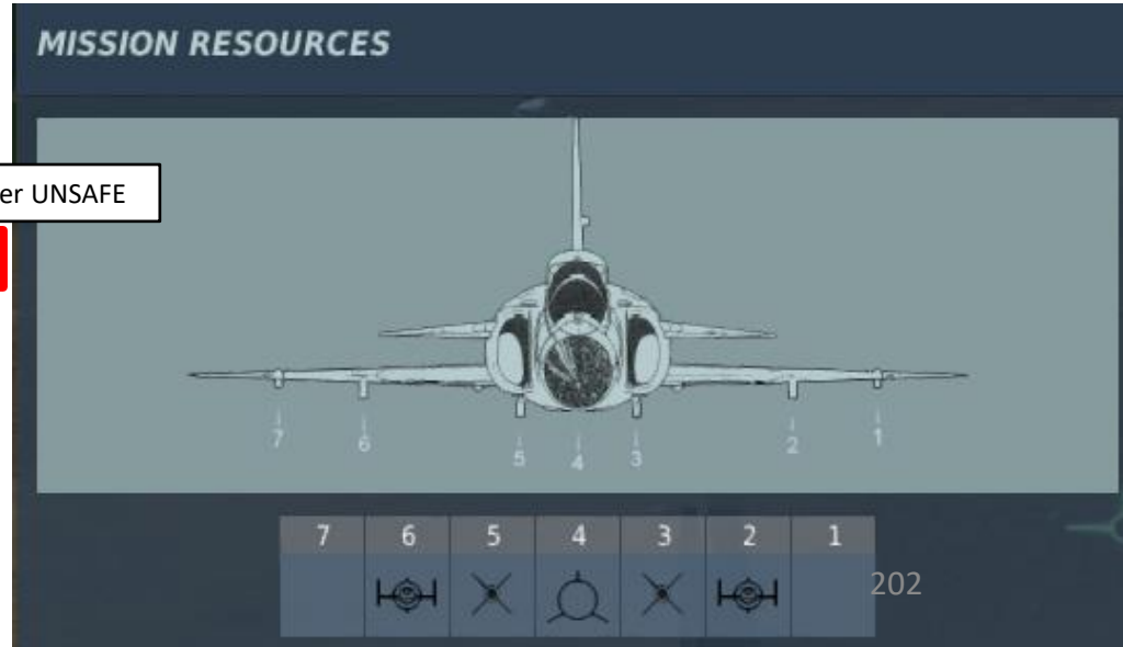
Weapon Status Codes: • 1 : Indicates that the pylon has a weapon attached and the weapon is fully functioning and ready to be used. • - : indicates the weapon has an error and is unusable. • 0 : Indicates that the weapon has been released. • Flashing : The currently Selected pylon is indicated by a flashing symbol.
